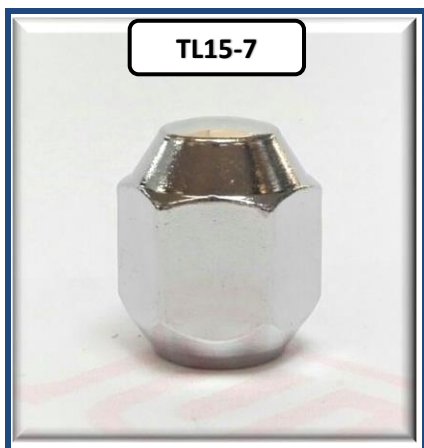
TUERCA LUJO, NISSAN 80, M12 X 1.25, HEXAGONO 21MM O 13/16", LARGA, ALTO 30MM
