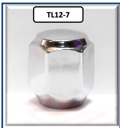
TUERCA LUJO, CHEV. SWIFT, M12 X 1.25, HEXAGONO 19MM O 3/4", ALTO 24MM
