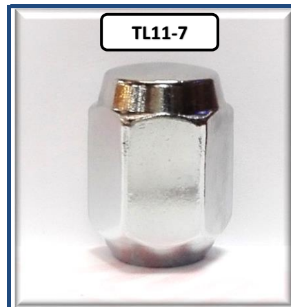
TUERCA LUJO, SUZUKI, M12 X 1.25, HEXAGONO 21MM O 13/16", ALTO 35MM
