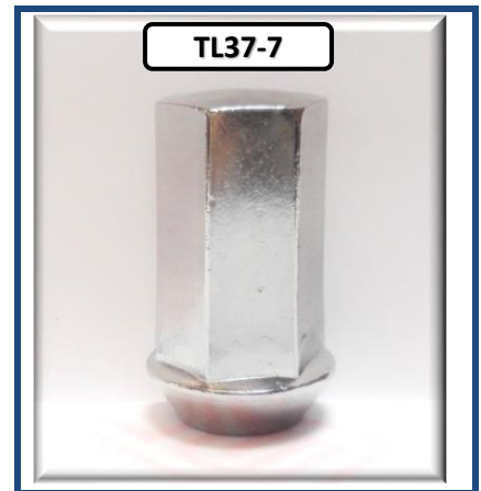
TUERCA LUJO, NISSAN MT3000, M16 X 1.50 X 55, ESTRIADA 2 LINEAS, HEXAGONO 22MM O 7/8", ALTO 56MM
